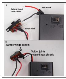
A.Cut at 1", trim and tin the Red and Black wires coming from the battery holder and add heat shrink both wires.
