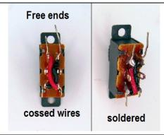
The switch is prepared by first soldering the two crossover wires to the end pins leaving some bare wire free at one end for connection to the battery. Bending out the middle pins will help seat these crossover wires
