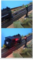
4. The Signal is connected to the green plug on the board via two connecting wires. There is no need for a resistor on the wire as the resistors required are located on the circuit board. The wires are attached to the plug so that the green LED is lit when the signal is in ready mode.
