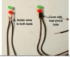
Cut two pieces of 8 inch black solid, 26 or 28 G wire. Solder the ends to the LED leads. Cover the joints with a short piece of 2mm heat shrink tubing and shrink using hot air.
