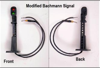
The wires at the back of the LEDs are painted black or covered with black putty. A 680 ohm is added to the one of the wires to limit the current to the LEDs and heat shrink is used to partly cover the body..
