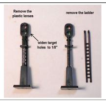
**Prep Signal** Remove the jewels and ladder from the signal stand. Widen the target openings to 1/8" diameter Widen two ladder holes in the base to 1/16 ".
