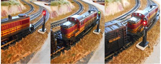
In this example the loco is stopped at the red light. Once the signal is switched to green the loco moves forward at which stage the switch turns is turned back to red
