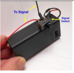
Heat shrink the joints and glue the switch to the body of the battery casing toward the front to avoid interfering with battery access. One could position the switch elsewhere just by extending the battery wiring.
