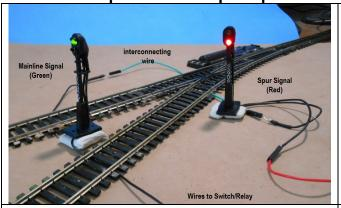
Set up for operating 2 Signals on a spur or cross over, The mainline signal is set to green The green wire connects to the spur signal set to red. This system will work for both the manual and automatic version.
