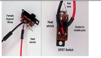
The Female Dupont wires have a short piece of heat shrink applied before soldering to the middle pins. Attach the red wire on the same side as the far red. Note the free exposed wire for connection to the battery wires.
