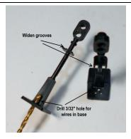
Drill a hole in the base behind the stand 3/32" in diameter for the wires to exit. Use a pilot drill first. Using a file or snippers widen the groove on the ladder support to accommodate the wires and the ladder.
