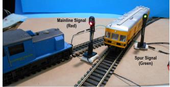
Here the Trolley the spur signal has been changed from red to green thus turning the mainline signal red to stop the oncoming diesel. After the time delay the spur signal goes red and the mainline turns green.
