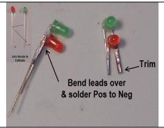
**LED Prep** Align Green over red polarity opposed . Solder the leads together . Trim to about ½ of lead length. If you test the lighting use only a 3V battery.
