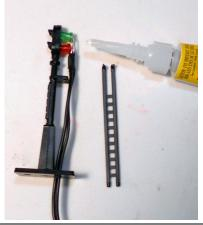
Insert the LEDs into the target holes. The LEDs can be glued in place with CA glue. Thread the wires down through the hole in the base. Reattach the ladder to the base holes and stem of the signal. Glue is used to secure the ladder in the holes and at the top.
