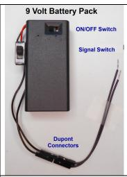
The Dupont connectors are linked up by aligning the open slits. The free end will be connected to wiring going to the signal. The Dupont connections allow for disconnection of the signal from the power source.
