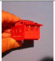
Two holes (5/64") are drilled into the rear wall just under the roof to fit the two red 2mm LEDs. These should fit snugly into the 2 holes.
