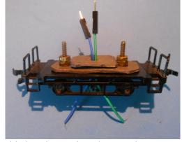
Weight is added to the truck and secured to ensure good track contact. These weights could have been secured with Blue Tack putty instead of the bolts. Two pick up wires are shown here, stripped and tinned and inserted through a hole drilled through the floor of the caboose.
