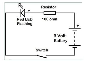
The circuit is setup as shown here using the flashing LED, 100 ohm resistor, 3 Volt battery in holder and a switch. Heat shrink tubing is used to prevent any short circuit. Cover the solder joints and heat with a heat gun or air dryer set on high.
