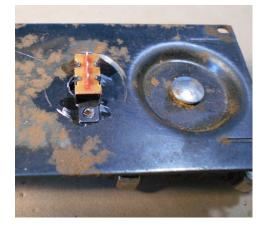
Remove any old rust, debris or spurs and sand the floor the floor flat. The switch is glued into place using a small amount of CA Super Glue make sure the slide moves freely in the hole before and after glueing.
