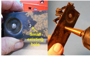
The switch will be inserted into a hole in the floor. Many pieces of rolling stock have a small hole that can be used or widened using a reaming drill bit. The hole should be around 5/16" in in diameter.
