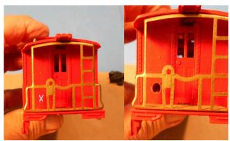
Select a spot where the Flashing End of Train (EOT) will be set. Drill a small pilot hole and expand this to 5/32" in diameter to allow the LED to pass through...
