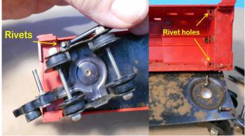
This American Flyer S Scale Caboose is secured by rivets at each corner of the floor. The rivets are lifted by heating with a solder iron then prying out of the holes using a flat screwdriver and long nose pliers
