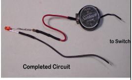
The lighting circuit is setup as shown. Shorten the LED leads to around 3/4", keeping the anode positive lead slightly longer. Shorten the **resistor** leads to about 1/2" on both sides. Solder the resistor to the anode (Positive) lead of the LED.
